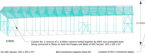
Bolt Connection Capacity check for combined tension and shear:  $ft/Pt + fs/Ps \le 1.4$  [Cobb 241] In this case shear controls:  $fs/Ps \le 1.4$
