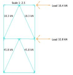
DESIGN all Struts and Ties to match Brace D; 6.7m in length @ 48.35 kN in Compression:
